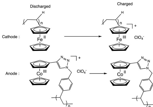
**Scheme 10** Electrode reactions in a recent RFBs based on ferrocene polymer as catholyte and cobaltocenium salt as anolyte (driving force: 1.3 V). Electrons are transported by  $\text{ClO}_4^-$  anions.
