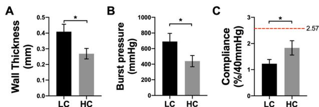
**Fig. 2** Mechanical properties of low compliance (LC) grafts and high compliance (HC) grafts. (A) Wall thickness, (B) burst pressure, and (C) compliance of LC and HC grafts.  $n = 3$ , \* indicates a significant difference using *t*-test with  $p < 0.05$ . Red dash line indicates the compliance of native rabbit carotid artery.
