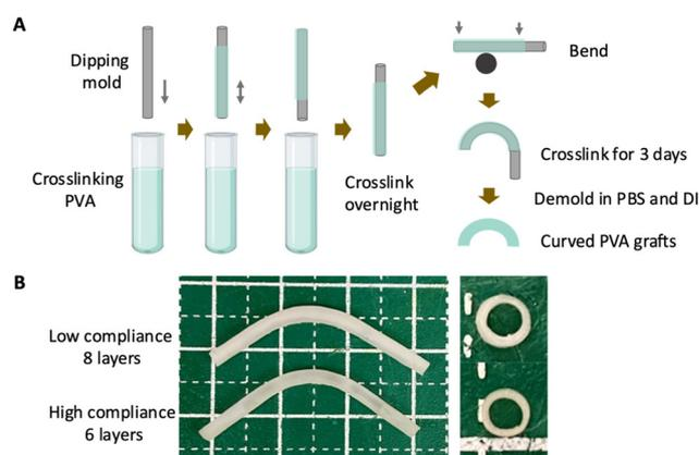
**Fig. 1** Fabrication of PVA small diameter vascular grafts with low compliance (LC) and high compliance (HC). (A) Schematic diagram of PVA small diameter vascular graft fabrication procedure. (B) Representative pictures of low compliance and high compliance PVA grafts.
