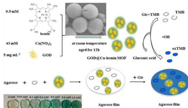
Fig. 9 Schematic of the peroxidase-like activity of the MOF and how the MOF-hydrogel film can be used to detect different concentrations of glucose by colorimetry. Reproduced with permission from ref. 69. Copyright 2021 Elsevier.
