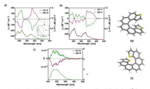
Fig. 3 The experimental UV-vis (bottom) and ECD (top) spectra of the (P) and (M) isomers of 10 and 11 (CH<sub>2</sub>Cl<sub>2</sub>,  $C \sim 10^{-5}$  M) are shown in panels (a and b), respectively. The inset in (a) shows the magnified ECD of (P) and (M)-10 in the 400-450 nm region. The fluorescence (bottom) and CPL (top) spectra of (P) and (M)-10 are shown in panel (c).
