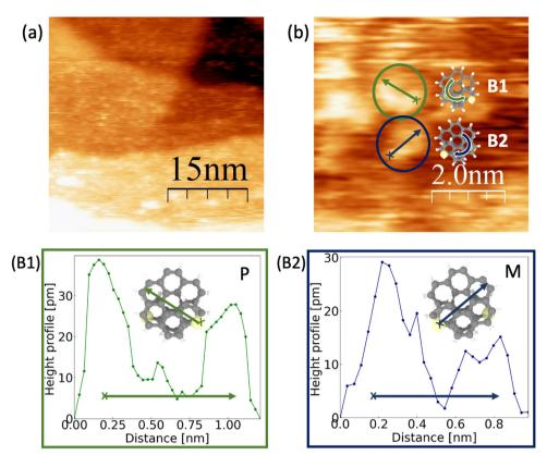
Fig. 9 Panel (a) shows a topographic image of exo-dithia[9]helicene acquired using  $V_{\text{bias}} = 0.5 \text{ V}$  and  $I_{\text{t}} = 0.1 \times 10^{-9} \text{ A}$ . (b) Zoomed in image of two enantiomer with chirality P in green and M, in blue, and the corresponding height profiles for each enantiomer (B1 for P and B2 for M). The set parameters were  $V_{\text{bias}} = 0.4 \text{ V}$  and  $I_{\text{t}} = 0.1 \times 10^{-9} \text{ A}$ .
