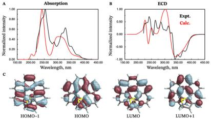
Fig. 8 Experimental (black curves) and calculated (red curves) absorption (panel A) and ECD (panel B) spectra of (M)-endo-dithia[7]helicene 11. Isosurfaces (±0.03 au) for the most relevant frontier molecular orbitals (HOMO-1, HOMO, LUMO, and LUMO+1) are shown in panel C. The calculated energies were shifted by -0.40 eV prior to conversion to wavelengths.
