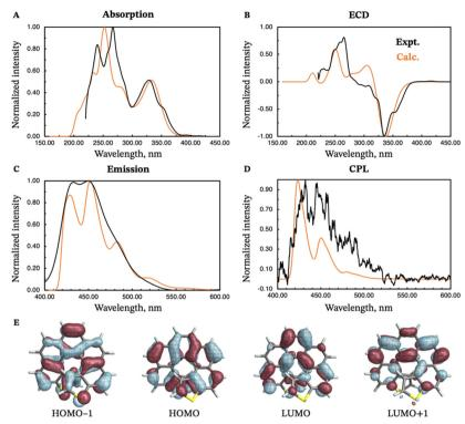
Fig. 7 Experimental (black curves) and calculated (orange curves) absorption (panel A), ECD (panel B), emission (panel C) and CPL (panel D) spectra of (M)-exo-dithia[7]helicene 10. Isosurfaces (±0.03 au) for the most relevant frontier molecular orbitals (HOMO-1, HOMO, LUMO, and LUMO+1) are shown in panel E. The calculated energies were shifted by -0.40 eV prior to conversion to wavelengths.
