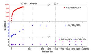
Fig. 5 Response changes of Cs<sub>4</sub>PbBr<sub>6</sub>/FAU-Y, Cs<sub>4</sub>PbBr<sub>6</sub>/SiO<sub>2</sub>, Cs<sub>4</sub>PbBr<sub>6</sub> NPs, and Cs<sub>4</sub>PbBr<sub>6</sub> LPs upon exposure to 45% RH condition.
