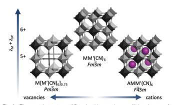
Fig. 1 The crystal structure of Prussian blue analogues. If the charges of the transition metals  $(z_{\rm M}+z_{\rm M'})$  sum to 6, the ordered MM'(CN) $_{\rm 6}$  is formed. For lower charges, vacancies or A-site cations are included to give the formulae  $M[M'(CN)_6]_{y<1}$  and  $A_{x>0}M[M'(CN)_6]$ , respectively. M is shown in dark grey, M' in light grey and A in purple.
