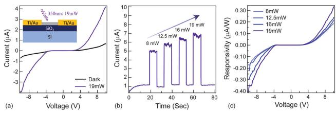
Fig. 5 Photoconductivity of NAI-TPE-PyS. (a) current vs. voltage measurements of the device. Inset: Schematic of NAI-TPE-PyS-coated two-terminal device.  $SiO_2$ :2  $\mu$ m; Ti: 5 nm; Au: 100 nm. Device channel size: length  $\times$  width = 200  $\mu$ m  $\times$  5000  $\mu$ m. (b) current vs. time measurements of the device at different incident optical powers. (c) Responsivity vs. voltage of the device at different incident optical powers.
