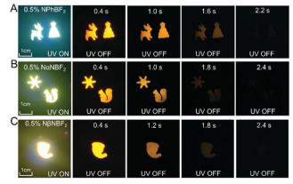
Fig. 2 Photographs of (A) NPhBF<sub>2</sub>-MeOBP-0.5%, (B) NαNBF<sub>2</sub>-MeOBP-0.5% and (C) N $\beta$ NBF<sub>2</sub>-MeOBP-0.5% afterglow materials under 365 nm UV light and after removal of the UV light.
