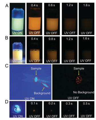
Fig. 7 (A) and (B) Photographs of (A)  $N\beta NBF_2-MeOBP-0.5\%$  and (B) NβNBF<sub>2</sub>-MeOBP-0.5% + R6G afterglow dispersion under 365 nm UV light and after removal of the UV light. (C) and (D) Preliminary bioimaging studies of the NBNBF2-MeOBP-0.5% afterglow dispersion in living (C) fish and (D) mice.
