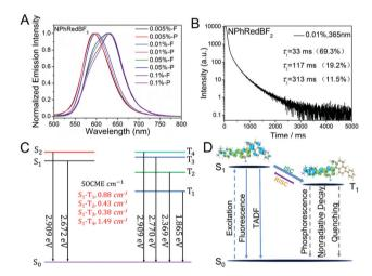
Fig. 4 (A) Room-temperature steady-state emission and delayed emission spectra of NPhRedBF2-MeOBP afterglow materials at different doping concentrations. (B) Room-temperature emission decay of NPhRedBF2-MeOBP-0.01% afterglow materials excited at 365 nm and monitored at 599 nm. (C) and (D) Schematic representations of (C) energy levels and spin orbital coupling matrix elements and (D) the proposed mechanism of organic afterglow in the NPhRedBF2-MeOBP system.
