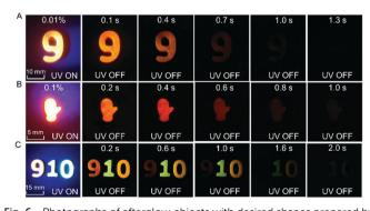
Fig. 6 Photographs of afterglow objects with desired shapes prepared by melt casting technique of (A) NPhRedBF2-MeOBP-0.01%, (B) NPhRedBF2-MeOBP-0.1% and (C) (left-right) NPhRedBF2-MeOBP-0.01%, N $\alpha$ N-MeOBP-0.5% and N $\beta$ NBF $_2$ -MeOBP-0.5% under 365 nm UV light and after removal of the UV light.
