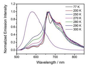
Fig. 5 Temperature-dependent delayed emission spectra NPhRedBF<sub>2</sub>-benzophenone samples.
