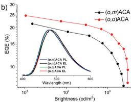
Fig. 3 OLED performance of D-A-D materials: (a) I-V curves with device stack inset. (b) EQE curves with EL and PL spectra inset.
