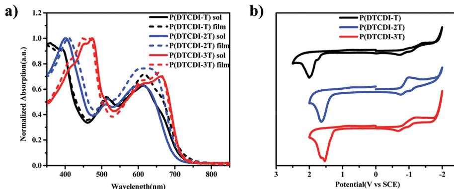
Fig. 1 (a) Optical absorption spectra of P(DTCDI-T), P(DTCDI-2T) and P(DTCDI-3T). (b) Cyclic voltammograms of P(DTCDI-T), P(DTCDI-2T) and P(DTCDI-3T) thin films measured in 0.1 M  $\text{Bu}_4\text{N}^+\text{PF}_6^-$  acetonitrile solution with a scan rate of  $100 \text{ mV s}^{-1}$ .
