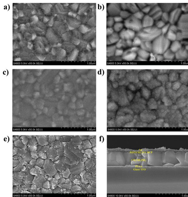
**Fig. 3** The SEM images of (a) MAPbI<sub>3</sub>, (b) MAPbI<sub>3</sub>/PCBM, (c) MAPbI<sub>3</sub>/P(DTCDI-T), (d) MAPbI<sub>3</sub>/P(DTCDI-2T), (e) MAPbI<sub>3</sub>/P(DTCDI-3T) and (f) cross-section of ITO/PTAA/MAPbI<sub>3</sub>/P(DTCDI-2T)/BCP/Ag.
