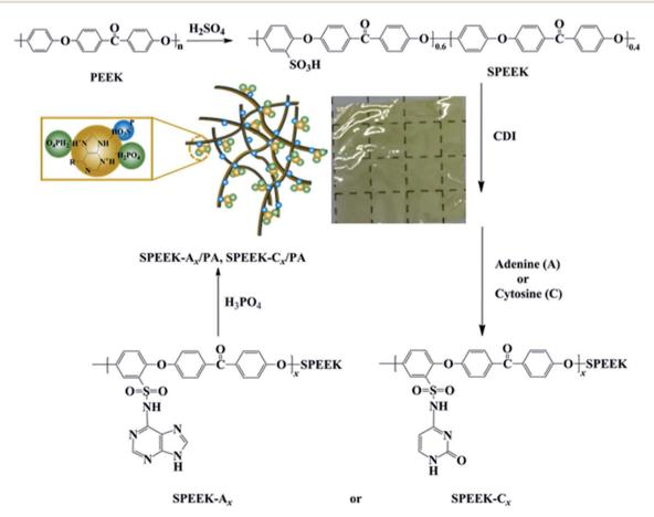
Scheme 1 Preparation of PA doping SPEEK-A<sub>x</sub> and SPEEK-C<sub>x</sub> membranes.
