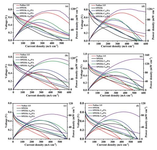
Fig. 6 Polarization and power density curves of SPEEK, SPEEK-A<sub>x</sub>/PA (a-c), SPEEK-C<sub>x</sub>/PA (d-f) and commercial Nafion 115 membranes with 1 M (a and d), 2 M (b and e), and 5 M (c and f) methanol as the fuel at 80  $^{\circ}$ C (methanol fuel with a flow rate of 1 mL min<sup>-1</sup> and oxygen with a flow rate of  $30 \text{ mL min}^{-1}$ ).
