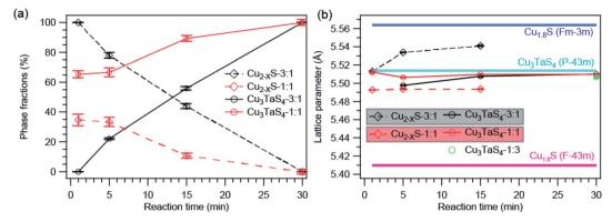
Fig. 3 Analysis from Rietveld refinement profile. (a) Phase fractions of  $Cu_{2-x}S$  and  $Cu_3TaS_4$  as a function of reaction time. (b) The calculated lattice parameters of  $Cu_{2-x}S$  and  $Cu_3TaS_4$  compared with standard lattice parameters of  $Cu_{1.8}S$ ,  $Cu_{1.6}S$ , and  $Cu_3TaS_4$
