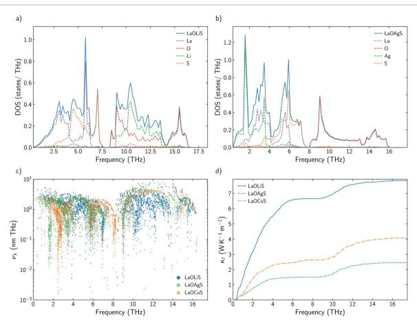
Fig. 5 (a and b) Total and projected phonon density of states, DOS, of LaOLiS and LaOAgS. (c) Group velocities,  $v_{\lambda}$  for LaOLiS (blue), LaOCuS (green), and BiOCuS (orange). (d) Cumulative κ<sub>1</sub> for LaOLiS (blue solid line), BiOAgS (green dashed line) and BiOCuS (orange dashed line).
