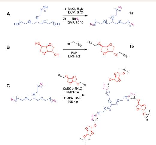
Scheme 1 Synthetic protocols employed in the preparation of (A) triazide glycerol ethoxylate and (B) bis-alkyne isosorbide derivates. (C) Synthesis of hydrogel films via Cu(i) mediated photo-click reaction
