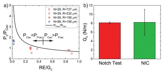
Fig. 4 (a) Plot of the experimentally observed critical expansion pressure  $P_c$  normalized by  $P_{Cav}$  against RE/ $G_c$ . The black line represents the point at which fracture is predicted to occur. (b) Plot showing the comparison between  $G_c$  measured with notch tests by Barney et al. 16 and measured with NIC in this work when RE/ $G_c \approx 0.84$ .
