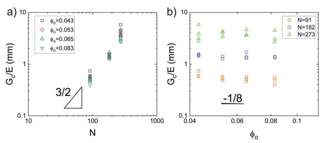
Fig. 2 Plots of the elastofracture length against (a) N and (b)  $\phi_o$  showing strong agreement with the scaling predictions of eqn (6). Data is taken from pure shear notch tests. Agreement between the data and theoretical scalings shows that altering N is a more effective means of tuning  $G_c/E$ .
