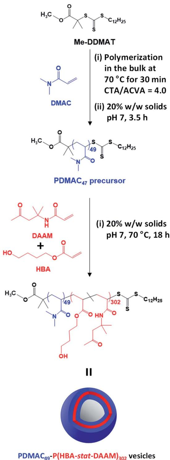
**Scheme 1** Reaction scheme for the synthesis of the PDMAC<sub>49</sub> precursor via RAFT aqueous solution polymerization of DMAC at 70 °C using a Me-DDMAT RAFT agent and an ACVA initiator. This PDMAC<sub>49</sub> precursor was subsequently chain-extended via RAFT aqueous dispersion copolymerization of a binary mixture of 80 mol% HBA and 20 mol% DAAM to produce PDMAC<sub>49</sub>-P(HBA-*stat*-DAAM)<sub>302</sub> vesicles at pH 7.
