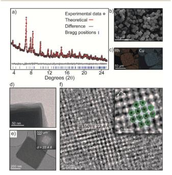
Fig. 3 (a) Rietveld refinement of the PXRD data of 3; (b) SEM image of 3 obtained from a DMF recrystallization; (c) EDX elemental mapping of Cu and Rh within crystals of 3; TEM images of 3 (d) the edge of a crystal, showing misalignment of layers; (e) the FFT pattern of a selected crystal; (f) an enlarged image of the same crystal showing the superimposition of the crystal structure of  ${\bf 3}$  along the c axis.
