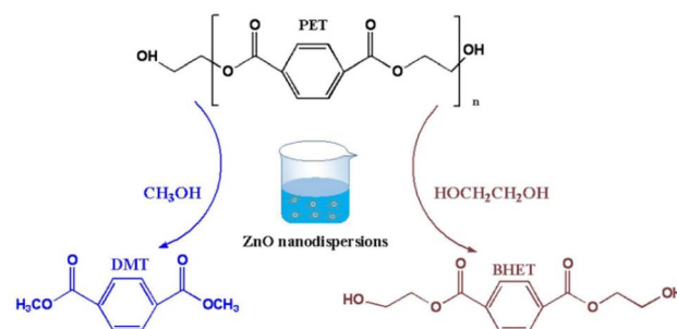
Fig. 11 Nano-ZnO dispersion catalyzed depolymerization of PET.
