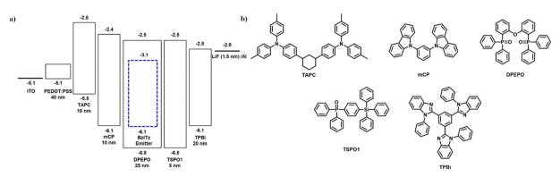
Fig. 5 (a) Device structure and energy-level alignment of the materials, and (b) chemical structure of the materials.
