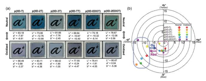
Fig. 2 (a) Photos of the fabricated ECD polymers p(IID-T), p(IID-3T), p(IID-T), p(IID-T), p(IID-EDOT) and p(IID-2EDOT) in the neutral and oxidised states (at +2.0, +2.0, +1.9, +1.9, +1.9 and +1.6 V, respectively), with their respective  $L^*$ ,  $a^*$  and  $b^*$  colour coordinates provided. (b) 2D colour chart of  $a^*$  vs.  $b^*$  with plots of the six polymers in the neutral and oxidised states.
