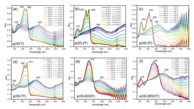
Fig. 1 Spectroelectrochemistry of isoindigo polymers (a) p(IID-T), (b) p(IID-2T), (c) p(IID-3T), (d) p(IID-TT), (e) p(IID-EDOT) and (f) p(IID-2EDOT) in fabricated ECDs, undergoing electrochemical oxidative doping.
