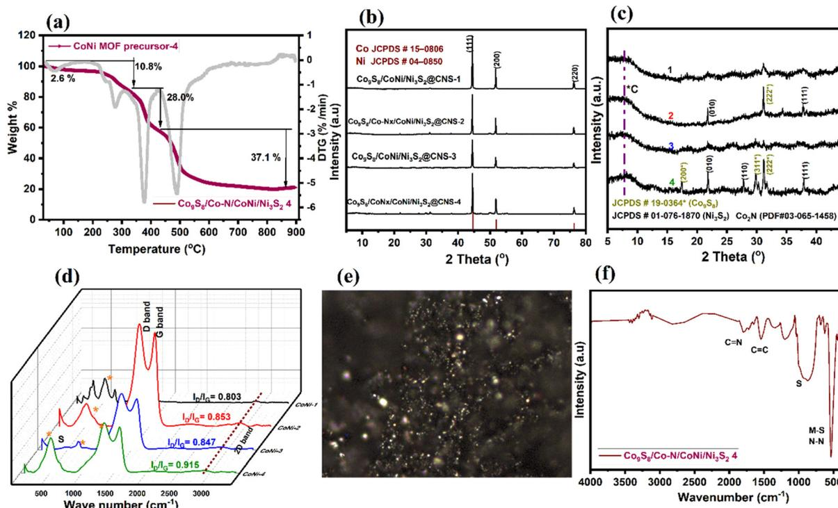
Fig. 4 (a) TGA spectrum of MOF precursor-4 conversion to catalyst  $\text{Co}_9\text{S}_8/\text{Co-N}_x/\text{CoNi/Ni}_3\text{S}_2@\text{CNS-4}$ , (b and c) XRD patterns of electrocatalysts  $\text{CoS/Co-N}_x/\text{CoNi/Ni}_3\text{S}_2@\text{CNS-1}$ –4, (d) Raman spectra of catalysts 1–4, (e) Raman image (laser at 532 nm) of a filter showing the distribution of graphitic carbon, and (f) the FT-IR spectrum of  $\text{Co}_9\text{S}_8/\text{Co-N}_x/\text{CoNi/Ni}_3\text{S}_2@\text{CNS-4}$ .
