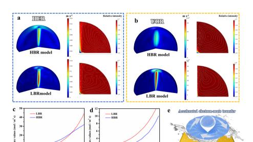
Fig. 6 (a) 3D and corresponding 2D simulation images of the microenvironment flow field states for the HBR and LBR models under the (a) HER and (b) UOR. (c and d) Comparison of the calculated transfer rates. (e) Schematic illustration of the optimal GMP mechanism.
