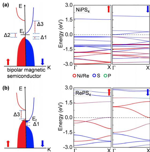
**Fig. 3** Electronic band structures of (a) NiPS<sub>4</sub> and (b) RePS<sub>4</sub> nanowires. The contributions from different atoms or orbitals are shown by the colors. The Fermi level is shifted to zero (red dashed lines). The left panels are schematic plots of their band structures.
