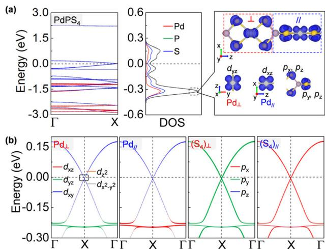
**Fig. 4** (a) Electronic band structures and density of states (DOS) of a PdPS<sub>4</sub> nanowire calculated without SOC. The right panel displays the partial charge density of the flat band at about  $-0.3$  eV. (b) Band structure of a PdPS<sub>4</sub> nanowire calculated with SOC. The contributions from different atoms or orbitals are shown by the colors. The Fermi level is shifted to zero (dashed lines).
