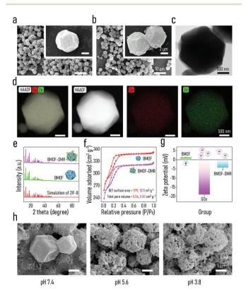
Fig. 1 SEM images of (a) BMOF and (b) BMOF-DMR (the green particles represent GOx); (c) TEM images and (d) elemental mapping of the BMOF; (e) XRD patterns and (f) N<sub>2</sub> adsorption-desorption isotherms of the BMOF and BMOF-DMR; (g) zeta potentials of the BMOF, GOx, and BMOF-DMR; (h) SEM images of the BMOF morphology after immersion in PBS with different pH values (37 °C, pH 7.4, 5.6, 3.8) for 7 d.
