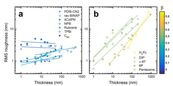
Fig. 2 Root mean square roughness versus film thickness for materials considered in this work and from literature. The data are separated for clarity with the materials that remain smooth (lower  $\beta$ ) in (a) and materials that become rough (higher  $\beta$ ) in (b). The color of each data set corresponds the slope of the fit line, which is equal to the growth exponent,  $\beta$ .
