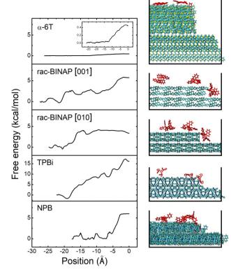
Fig. 4 Trajectories of  $\alpha$ -6T, rac-BINAP, TPBi and NPB molecules during a step-edge descent and their respective free energy profiles. The molecule's position at the step-edge after descent corresponds to 0 Å. For rac-BINAP the trajectories in both the [010] and [001] directions are shown.
