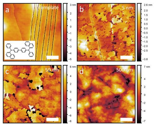
Fig. 1 Atomic force microscope images of an (a) NPB template crystal and (b) 5 nm, (c) 50 nm and (d) 500 nm of additional NPB grown on top of the template. Scale bars are 1 µm. Molecular structure of NPB is shown as an inset in (a).
