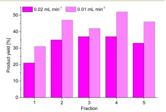
Fig. 10 Results for continuous catalysis of the Knoevenagel condensation between benzaldehyde and malononitrile using ZIF-8@Pine-APTES as catalyst. One fraction is equal to 1 mL of precursor solution pushed out of the syringe.
