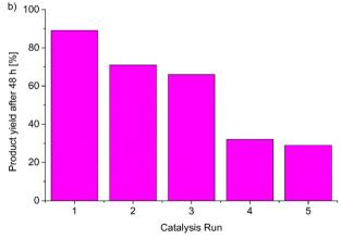
Fig. 9 a) Product yield from the Knoevenagel condensation between benzaldehyde and malononitrile catalyzed by ZIF-8@Pine-APTES or Pine-APTES including the blind test without catalyst. b) Product yield for the catalysis with ZIF-8@Pine-APTES after 48 h over 5 reaction cycles.
