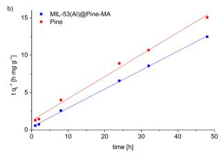
Fig. 7 a) Concentration of methylene blue as a function of time during the adsorption with MIL-53(Al)@Pine-MA and Pine. b) Linearized pseudo second order kinetics for the sorption of MB including the corresponding fitting curves (solid lines). As a result of the linearization, the material with faster sorption kinetics has a lower
