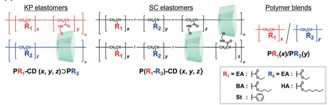
Fig. 2 Chemical structures of (a) the main chain monomers (EA, BA, HA, and St), the peracetylated CD monomer (TAcyCDAAmMe), (b) the primary polymers (PR<sub>1</sub>-PAc $\gamma$ CD (x, y)), (c) the KP elastomers (PR<sub>1</sub>-CD (x, y)) PR<sub>2</sub> (z)), the SC elastomers (P(R<sub>1</sub>-R<sub>2</sub>)-CD (x, y, z)), and the polymer blends  $(PR_1(x)/PR_2(y)).$
