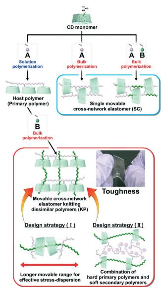
Fig. 1 Routes toward two different material designs with movable cross-links: single movable cross-network elastomer  $(SC)^{115,116}$  and movable cross-network elastomer for knitting dissimilar polymers (KP). KP elastomers allow for the two design strategies: (I) and (II).
