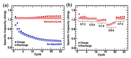
Fig. 15 (a) Specific capacity versus cycle number for a nanostructured Ge electrode cycled at a C/7.2 rate for 25 cycles; the data of the as-deposited Ge electrode cycled at the same rate is provided for comparison. (b) Specific capacity versus cycle number for the nanostructured Ge electrode cycled sequentially at C/7.2, C/3.6, C/1.8, C/0.9, and C/7.2 rates, respectively. Reproduced with permission from ref. 119. Copyright 2012, AIP Publishing.
