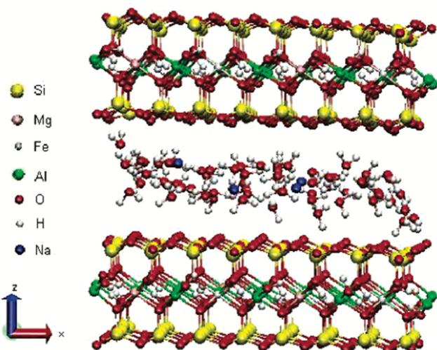
Fig. 3 Structure of Na-montmorillonite with two water layers.<sup>45</sup>
