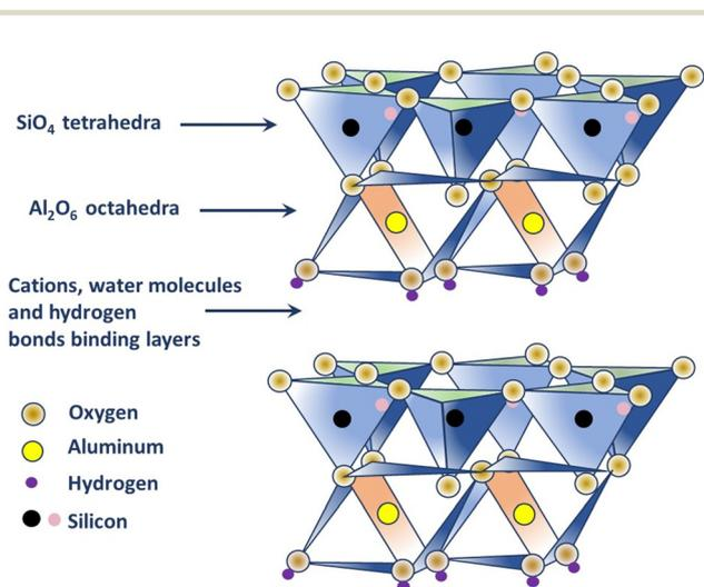
Fig. 1 Structure of kaolinite.
