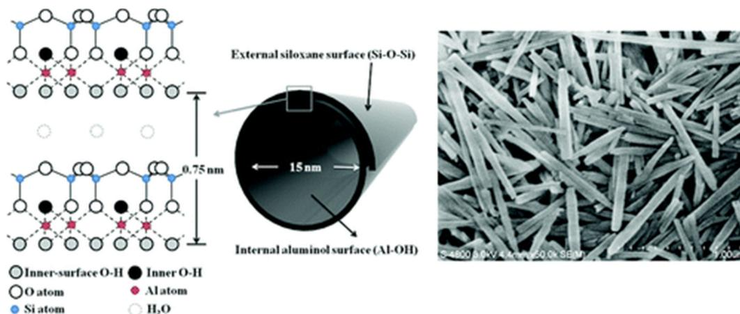
Fig. 2 Crystalline structure and FE-SEM image of halloysite nanotubes.<sup>40</sup>
