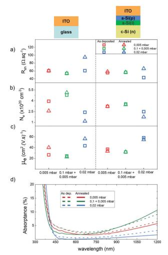
Fig. 2 (a) Sheet resistance  $(R_{sh})$ , (b) free carrier density  $(N_e)$  and (c) electron mobility ( $\mu_e$ ) of PLD ITO films deposited at LP (0.005 mbar); LP with buffer (0.1 + 0.005 mbar) and high pressure (0.02 mbar) on glass (left) and a-Si:H/c-Si stacks (right). (d) Absorptance as a function of wavelength of the ITO films.
