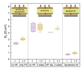
Fig. 6 Comparison of total series resistance ( $R_s$ ) for a set of SHJ cells with PLD ITO at the front and PLD or sputtered rear electrode and Ag grid pitch of 1 and 1.7 mm, respectively. R<sub>s</sub> of the cell with double-sided sputtered ITO is given for reference.
