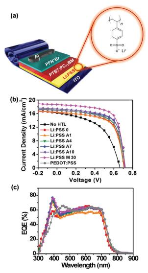
Fig. 2 (a) Device architecture of conventional OSCs with ITO/Li:PSS/ PTB7:PC<sub>71</sub>BM/PFN<sup>+</sup>Br<sup>-</sup>/Al and the chemical structure of Li:PSS, (b) J-Vcurves of PTB7:PC71BM OSCs measured under simulated AM 1.5G solar light and (c) EQE spectra.
