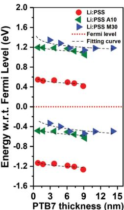
Fig. 7 Energy band structure relative to the Fermi level based on the changes in EA (top half) and IP (bottom half).
