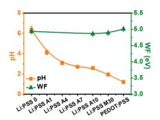
Fig. 1 pH values and work functions of Li:PSS and mixtures with PED-OT:PSS in various proportions
