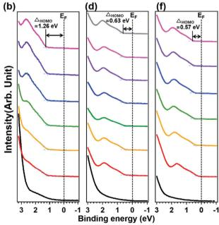
Fig. 5 UPS spectra for PTB7 films with different thicknesses on top of (a) and (b); Li:PSS A10 (c) and (d); and Li:PSS M30 (e) and Li:PSS (f) substrates. (a), (c), and (e) show the secondary edge while (b), (d), and (f) show the Fermi edge.
