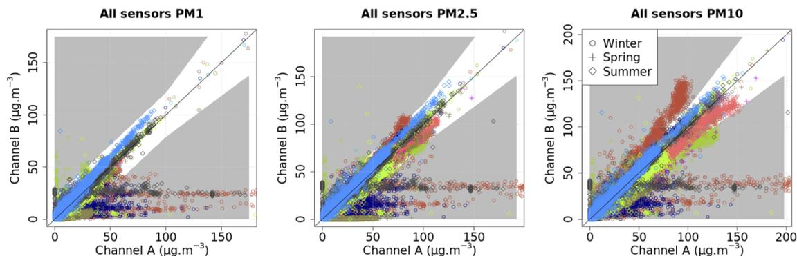
Fig. 1 Inter-channel performance of the PurpleAir systems for  $PM_1$ ,  $PM_{2.5}$  and  $PM_{10}$  (1 minute readings). Each color represents an individual system/campaign pair. The shaded areas represent measurements that do not meet the QA/QC criteria.
