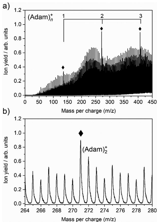
Fig. 1 (a) Time-of-flight mass spectrum of helium nanodroplets doped with adamantane, showing cationic adamantane clusters,  $(\text{Adam})_n^+$ ,  $n = 1-3$  (136, 272, and 408  $m/z$ ) along with their dehydrogenated analogues are also highlighted ( $\blacklozenge$ ). (b) Inlet between 264–280 mass units to highlight the cationic adamantane dimer and its dehydrogenated analogue at 272 and 271  $m/z$ , respectively.
