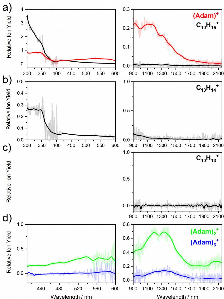
Fig. 2 Absorption spectra of (a)  $(\text{Adam})^+$  and its dehydrogenated analogue, (b) the doubly dehydrogenated analogue,  $\text{C}_{10}\text{H}_{14}^+$ , (c) the triply dehydrogenated analogue,  $\text{C}_{10}\text{H}_{13}^+$ , and (d) the adamantane dimer, and trimer cation,  $(\text{Adam})_2^+$  and  $(\text{Adam})_3^+$ . In each case, the spectrum is recorded by monitoring the increase in ion signal of the “bare” ion mass.
