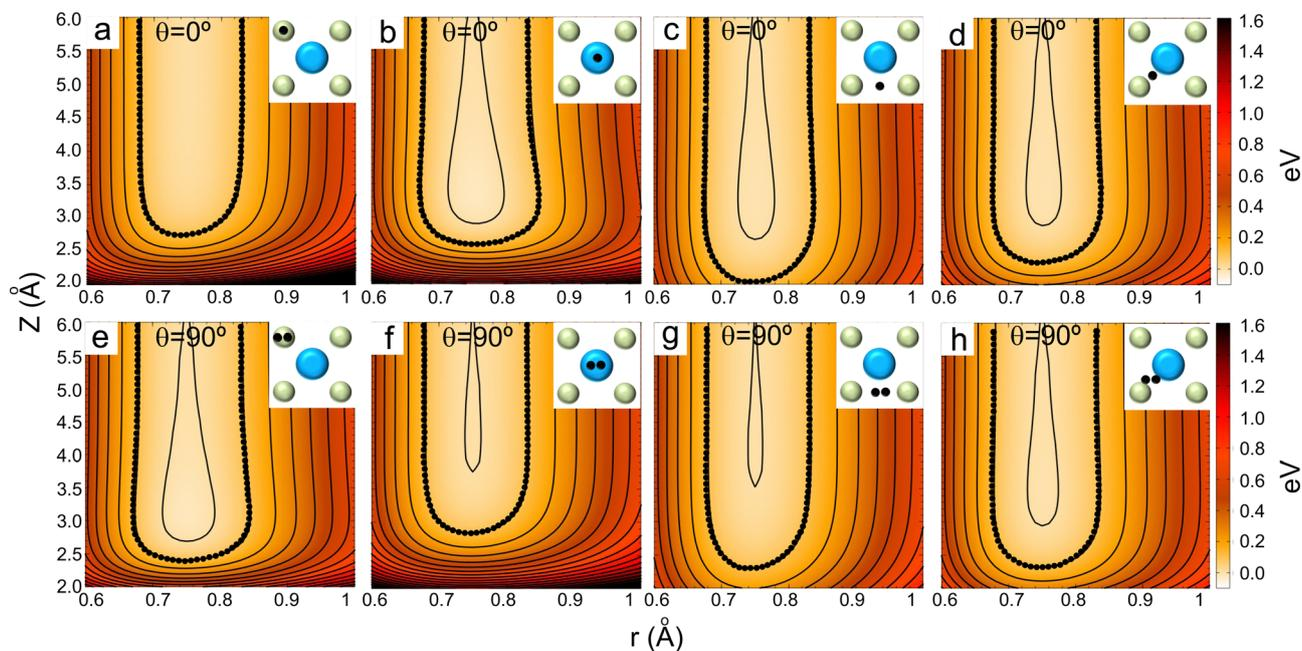
**Fig. 2** 2D cuts through the  $H_2/KCl(001)$  6D PES. Top panels: Cartwheel configurations; bottom panels: helicopter configurations. From left to right: Top K, top Cl, K–K bridge, and K–Cl bridge. The spacing between the contour levels is 0.1 eV. The dotted lines show the 0.1 eV isovalue. Blue balls represent Cl atoms, green balls K atoms, and black balls H atoms.
