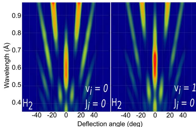
Fig. 4 Simulated  $\text{H}_2/\text{KCl}(001)$  GIFMD patterns along the crystallographic direction  $[100]$  for the initial rovibrational state: left panel ( $\nu = 0, J = 0$ ); right panel ( $\nu = 1, J = 0$ ).
