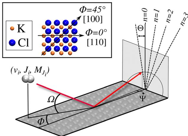
Fig. 3 Schematic representation of the diffraction process of  $\text{H}_2$  from a  $\text{KCl}(001)$  surface, with the projectile path represented in red. We indicate in the detection plane both the deflection angle  $\theta$ , and the diffraction order,  $n$ . The inset shows a top view of the surface, indicating the correspondence between  $\phi$  and the crystallographic direction.
