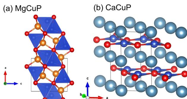
Fig. 1 Crystal structures of (a)  $\text{MgCuP}$  and (b)  $\text{CaCuP}$ . Mg = orange, Ca = turquoise, Cu = blue and P = red. In  $\text{MgCuP}$ , edge linked  $\text{CuP}_4$  tetrahedra form chains aligned in the  $b$  direction.
