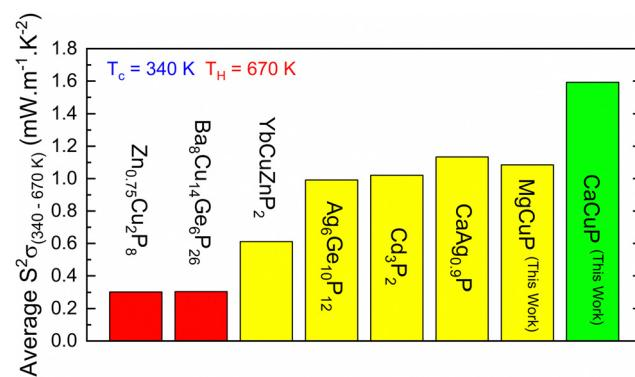
Fig. 4 Overview of temperature-average power factor  $\langle S^2/\rho \rangle$  for leading metal phosphide thermoelectrics. Data taken from:  $\text{Zn}_{0.75}\text{Cu}_2\text{P}_8$ ,<sup>11</sup>  $\text{Ba}_8\text{Cu}_{14}\text{Ge}_6\text{P}_{26}$ ,<sup>10</sup>  $\text{YbCuZnP}_2$ ,<sup>8</sup>  $\text{Ag}_6\text{Ge}_{10}\text{P}_{12}$ ,<sup>6</sup>  $\text{Cd}_3\text{P}_2$ ,<sup>13</sup>  $\text{CaAg}_{0.9}\text{P}$ ,<sup>14</sup> CaCuP (This Work).
