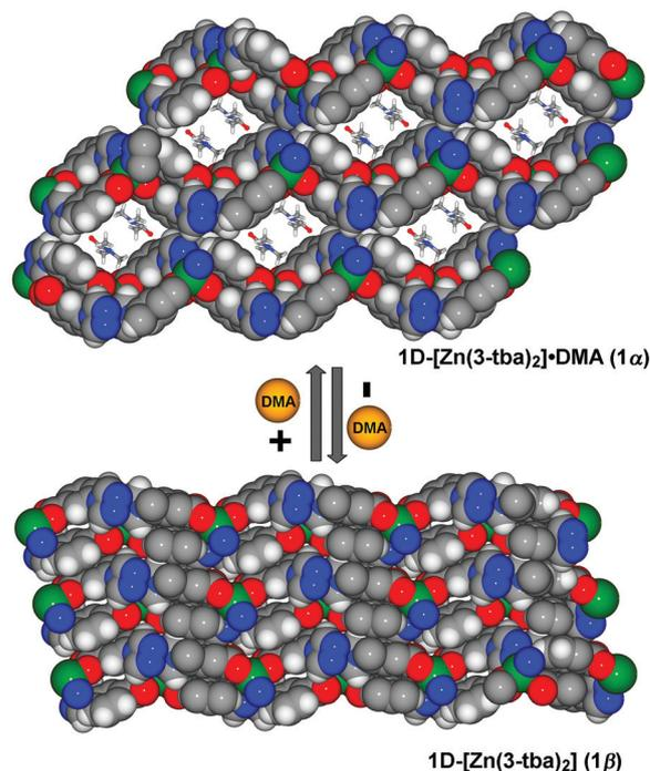
Fig. 2 Space-filling diagrams of the reversible structural transformation between  $1\alpha$  and  $1\beta$  (viewed along the *a*-axis, for more details see Fig. S5, ESI<sup>†</sup>).
