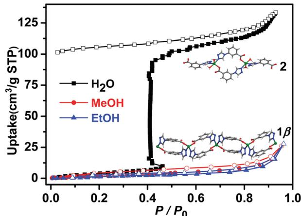
Fig. 4 Water, methanol and ethanol vapour sorption isotherms of  $1\beta$  collected at 298 K (closed and open symbols denote adsorption and desorption, respectively).
