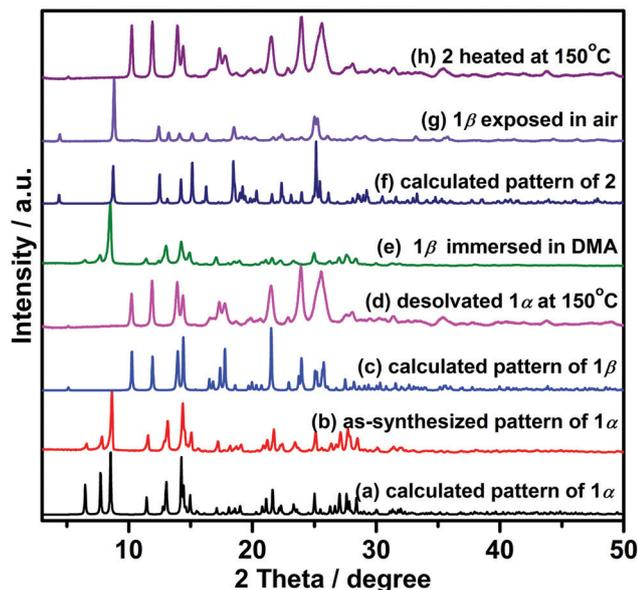
Fig. 3 PXRD patterns of (a)  $1\alpha$  calculated from SCXRD data, (b) as-synthesized  $1\alpha$  at room temperature, (c)  $1\beta$  calculated from SCXRD data, (d) desolvated  $1\alpha$  at  $150^\circ\text{C}$ , (e)  $1\beta$  immersed in DMA for 1 day, (f) calculated  $2$  from SCXRD data, (g)  $1\beta$  exposed to humid air (ca. 45% RH), and (h) dehydrated  $2$  at  $150^\circ\text{C}$ .
