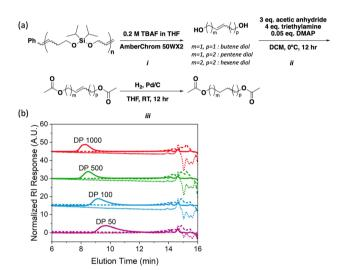
Fig. 2 Poly(iPrSi8) deconstruction and regiochemical analysis. (A) Quantitative fluoride-triggered deconstruction (i), acetylation (ii), and hydrogenation (iii) of poly(iPrSi8) to yield a mixture of protected saturated diols. (B) SEC traces (normalized RI) of poly(PrSi8) to different target DP (solid line, correlated to Table 2, entries 6-9) and subsequent deconstruction with 0.2 M TBAF in THF (dotted line) and 0.5 M HCl in dioxane (dashed line).
