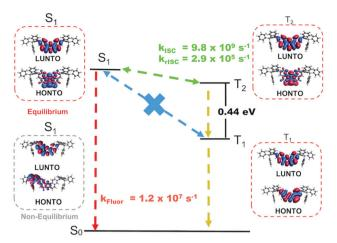
Fig. 5 NTOs for the  $S_1$ ,  $T_1$  and  $T_2$  states and schematics of the TADF mechanism in compound 1 with DFT estimated rates in toluene. A CT S<sub>1</sub> state calculated at a non-equilibrium geometry is also shown.
