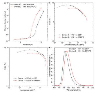
Fig. 4 Device characteristic
