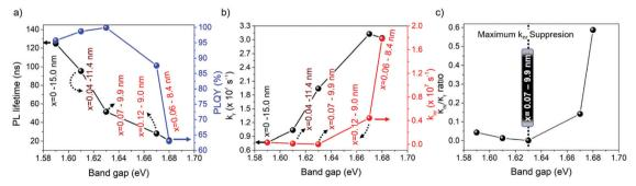
Fig. 5 (a) Behavior of the PL lifetime and PLQY, (b) radiative  $(k_r)$  and non-radiative recombination  $(k_{nr})$  decay rate constants, and (c) their corresponding  $k_{nr}/k_r$  ratio for the FAPb<sub>1-x</sub>Sr<sub>x</sub>l<sub>3</sub> PQDs colloidal solutions by varying the Sr fraction.
