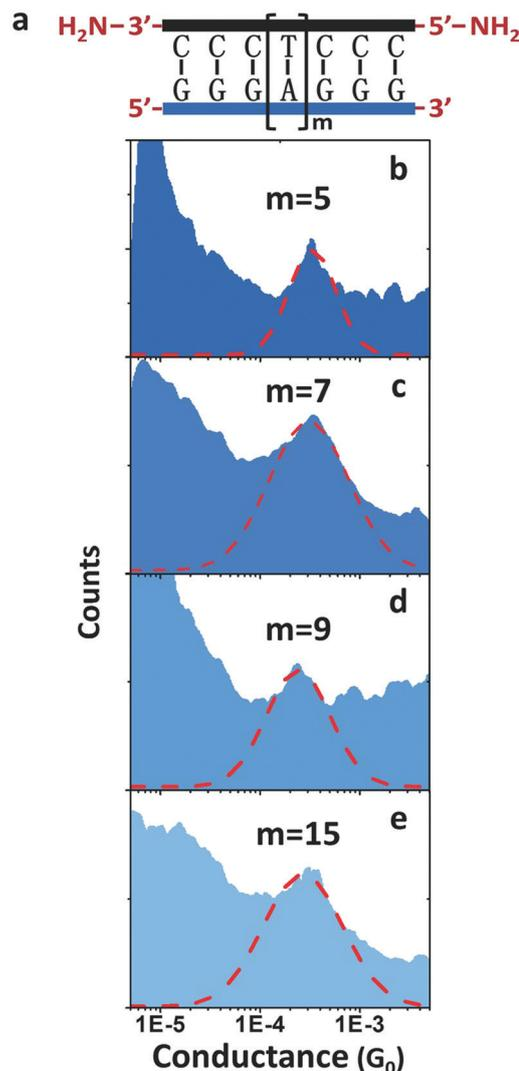
Fig. 5 DNA:RNA conductance in adenine-rich sequences. Conductance measurements of adenine-stacked RNA:DNA hybrids. (a) Illustration of the GGG-Am-GGG RNA:DNA hybrids. (b–e) Conductance histograms of four RNA:DNA hybrids ( $m = 5, 7, 9,$  and  $15,$  respectively). Red dashed line shows the Gaussian fitting of each peak. Reproduced with permission from ref. 73.
