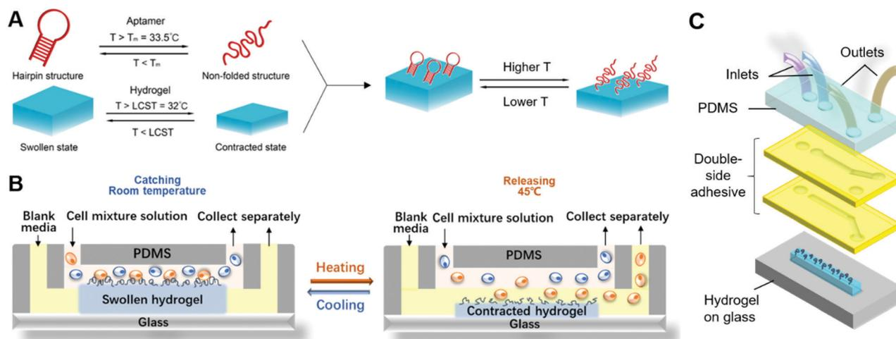
**Fig. 1** (A) The reversible response to the temperature of the aptamer, hydrogel and aptamer-functionalized hydrogel. (B) The cell separation mechanism of the iCatch microfluidic device consisting an aptamer-functionalized hydrogel placed in microfluidic channels. (C). The design of the iCatch consisting an aptamer-functionalized hydrogel placed in microfluidic channels with two inlets respectively leading to the upper and lower streams and two outlets.
