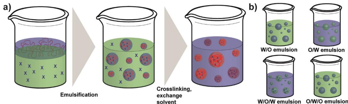
**Scheme 5** Schematic overview over the emulsion process for polysaccharide NP formation: (a) formation of polysaccharide NPs via water-in-oil emulsion and crosslinking (external gelation) and (b) types of emulsions used to prepare polysaccharide NPs (green: organic solvent; blue: water).
