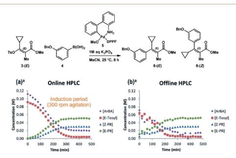
Fig. 18 Reaction monitoring with online HPLC analysis enables a more accurate reaction snapshot. Reproduced from ref. 36 with permission from the Royal Society of Chemistry.
