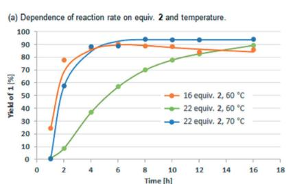
Fig. 17 DoE time course studies enabled by an acidic quench in the Vilsmeier Haack bromination of  $\gamma$ -cyclodextrin. Adapted with permission from ref. 31. Copyright 2021 American Chemical Society.
