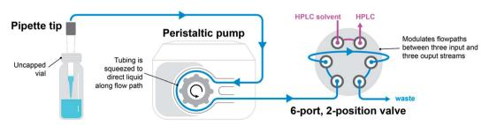
Fig. 4 Liquid handling modules arranged in two configurations: a syringe pump, selector valve, and needle tip (top) and a peristaltic pump, 6port, 2-position valve, and pipette tip (bottom).
