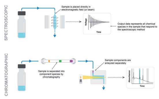
Comparison of simple spectroscopic (top) and chromatographic (bottom) analytical methods
