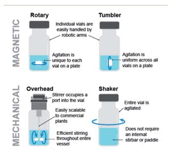
Fig. 6 Magnetic and mechanical stirring modules impart different agitation homogeneity across a reaction plate, efficiency, and scalability.
