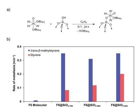
Fig. 6 (a) Preparation of well-defined silica-supported W(v) oxo species. (b) Rates of metathesis of trans- $\beta$ -methylstyrene (blue) and styrene (red) catalysed by W(IV) oxo species, molecular and supported on silica prepared at different dehydroxylation temperatures. Reprinted with permission from ref. 164. Copyright 2019 American Chemical Society.
