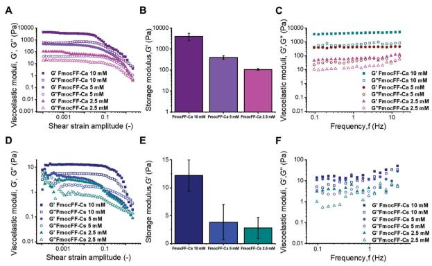
Fig. 5 Mechanical characterization of the samples under oscillatory shear. (A) and (C) show the amplitude and frequency sweeps for Ca<sup>2+</sup> samples, and (B) the mean and standard deviation of the storage modulus corresponding to the linear viscoelastic region. (D)–(F) show the same results but for Cs<sup>+</sup> samples.
