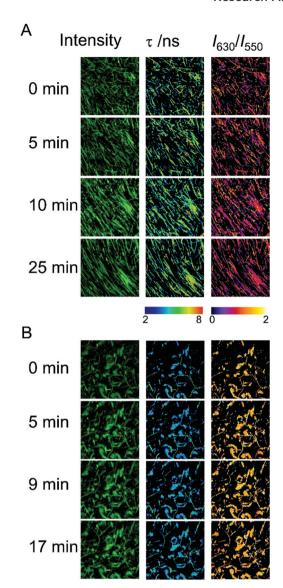
Fig. 6 Intensity, FLIM, and ratiometric images of the dye AQui in self-healing Fmoc-FF hydrogels formed with Ca<sup>2+</sup> (A) and Cs<sup>+</sup> (B) after ultrasound treatment, as a function of time. The size of the images is 10  $\mu m \times$  10  $\mu m$ .
