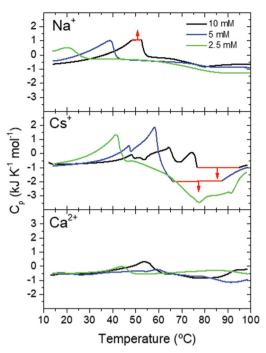
Fig. 4 DSC scans of Fmoc-FF at different concentrations in the presence of different cations. Thermogram regions in red indicate signal saturation of the calorimeter.
