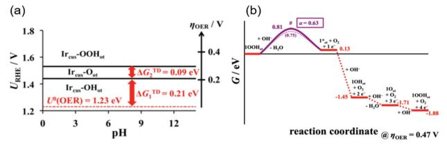
Fig. 5 Theoretical studies for OH<sup>-</sup> oxidation over iridium oxide. (a) The ab initio Pourbaix diagram for a single-crystalline IrO<sub>2</sub>(110). (b) The free energy diagram over IrO<sub>2</sub>(110) in alkaline media (pH = 12.9) at an OER overpotential of 0.47 V. Reprinted with permission from ref. 95. Copyright (2019) American Chemical Society.
