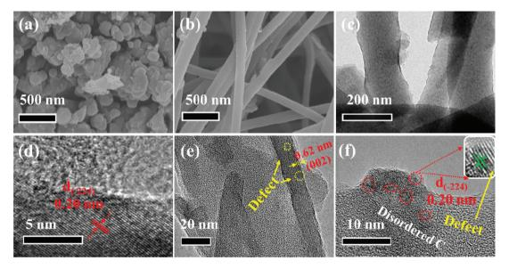
Fig. 1 SEM morphology of (a) P-V<sub>5</sub>S<sub>8</sub>/C and (b) D-V<sub>5</sub>S<sub>8</sub>/CNFs. (c) TEM image of D-V<sub>5</sub>S<sub>8</sub>/CNFs. The corresponding HRTEM images of (d) P-V<sub>5</sub>S<sub>8</sub>/C and (e and f) D-V<sub>5</sub>S<sub>8</sub>/CNFs. Note that the inset of (f) shows the relevant enlargement of the dashed box (red).
