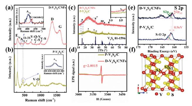
Fig. 2 (a and b) Raman spectra, (c) XRD pattern, (d) EPR spectrum, and (e) XPS analysis of the P-V<sub>5</sub>S<sub>8</sub>/C and D-V<sub>5</sub>S<sub>8</sub>/CNF samples. (f) Schematic illustration of the atom arrangements in  $V_5S_8$ ; note that S1, S2, and S3 represent the possible sulfur defects.
