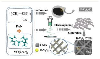
Scheme 1 Schematic illustration for synthesizing the D-V<sub>5</sub>S<sub>8</sub>/CNF and P-V<sub>5</sub>S<sub>8</sub>/C composites.
