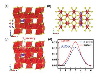
Fig. 7 The minimum energy path for the K atom diffusion pathways in (a and b)  $P-V_5S_8$  and (c) S-defective  $V_5S_8$ .<sup>17</sup> (d) The corresponding barrier energy. The yellow, red and purple balls represent the S, V and K atoms, respectively.
