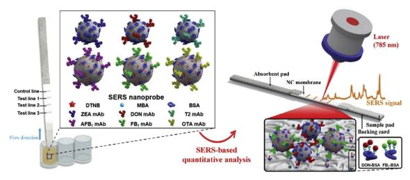
Fig. 5 Schematic of multiplex detection of mycotoxins using SERS-based lateral flow immunosensor. Reproduced with permission from ref. 75. Copyright 2020, Elsevier.
