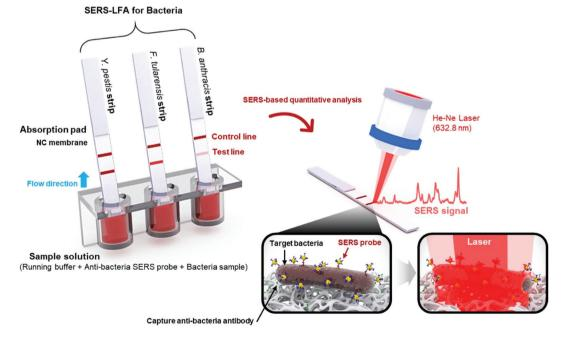
Fig. 11 Schematic representation of the experimental flow for detection of Y. pestis, F. tularensis and B. anthracis bacterial strains on the SERSbased LFA sensing platform. The immunocomplexes from bacteria and probe interactions travelled by capillary action towards the test line where SERS measurements were acquired and analysed. Reproduced with permission from ref. 139. Copyright 2017; Elsevier.
