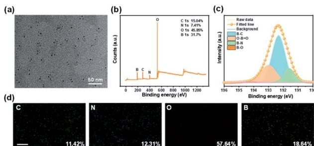
Fig. 2 (a) TEM image of CD/BNO. (b) XPS spectra of CD/BNO. (c) XPS high-resolution B 1s spectra of CD/BNO. (d) Energy-dispersive X-ray spectroscopy (EDS) mapping images of CD/BNO, scale bar is 5  $\mu\text{m}$ .
