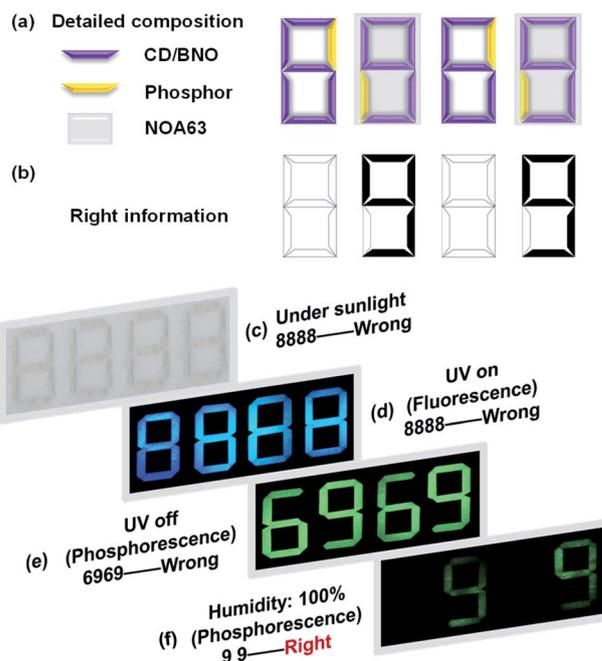
**Fig. 6** (a) Detailed composition of the patterned template. (b) Hidden right information. (c) Digital photos of a  $4 \times 7$  bar-shaped pixel matrix fulfilled by CD/BNO, CD phosphor and NOA63 (Norland Optical Adhesive 63) under sunlight. (d) Digital photos with UV on. (e) Corresponding images with UV off in different environments. (f) Demonstration of the anti-counterfeiting.
