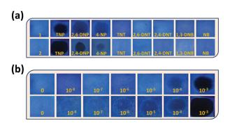
Fig. 10 (a) Paper strips encrusted with  $\bf 1$  (top) and  $\bf 2$  (bottom) and their respective visualisation in the presence of different NACs under UV light ( $\lambda=365$  nm). (b) Photographs of paper strips coated with  $\bf 1$  (top) and  $\bf 2$  (bottom) with increasing concentration of TNP ( $10^{-8}$  to  $10^{-3}$  M).
