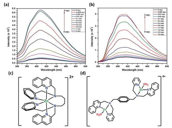
Fig. 12 Emission spectra of (a) 1 and (b) 2 (32 μM) in DMF: H<sub>2</sub>O (1:1) with an increase in concentration of Zn<sup>2+</sup> ranging from 0 to 64 μM and 0 to 96 μM, respectively ( $\lambda_{exc}$  = 340 nm). Schematic representation of 1:1 and 1:2 complex formation in the presence of one and two equivalents of Zn<sup>2+</sup> ion for 1 (c) and 2 (d), respectively
