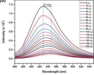
Fig. 2 Effect on the emission spectra of (a) 1 and (b) 2 dispersed in Milli-Q water (1 mg, 2 mL) upon incremental addition of TNP (1 mM) ( $\lambda_{exc}$  = 340 nm).
