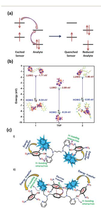
Fig. 6 (a) Schematic illustration of the quenching mechanism *via* photo-induced electron transfer. (b) Calculated energy diagram with the HOMO–LUMO energies of **1**, **2** and TNP. (c) Possible mechanism of TNP sensing in (i) **1** and (ii) **2**.
