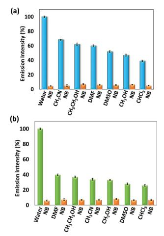
Fig. 1 Change in emission intensity % after addition of nitrobenzene to (a) 1 and (b) 2 in the presence of different solvents
