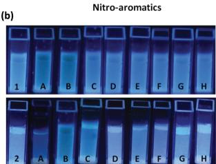
(a) Fluorescence quenching (%) of 1 and 2 dispersed in water (1 mq, 2 mL) by different NACs (200  $\mu$ L, 1 mM). (b) Cuvette photographs of **1** and **2** before and after the addition of 200 µL of different analytes upon UV-light illumination at  $\lambda$  = 365 nm, where, A: TNP; B: 2,4-DNP; C: 4-NP; D: 2,4-DNT; E: TNT; F: 2,6-DNT; G: 1,3-DNB; H: NB.
